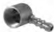
Art. 471EGN Raccordo portagomma femmina 90° per gas metano o gpl a norma UNI CIG-7129 in ottone nichelato Brass hose nipple 90° for natural gas or lpg in accordance with UNI CIG-7129 nickel plated
